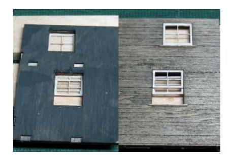
NOTE: You may notice in the photo, last column, proceeding page, that the outer edges of the window sills aren't painted. This is normal as it can't be done while they are attached to the carrier sheet. Wait until all the windows are installed then touch these edges up.
