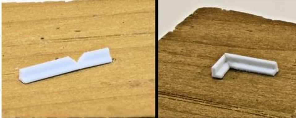
**Version 1** – I simply notched out part of the angle, bent it around and cemented to form a foot.
