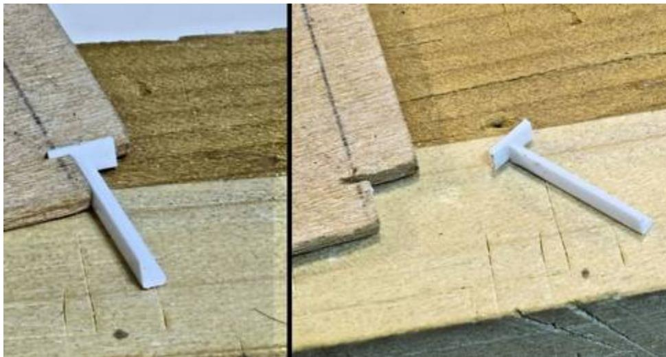
**Version 2** – Made a quick jig from some scrap balsa – a small slot to hold some flat-stock (not in the kit) and glued a length of the 1/16" angle to it.
