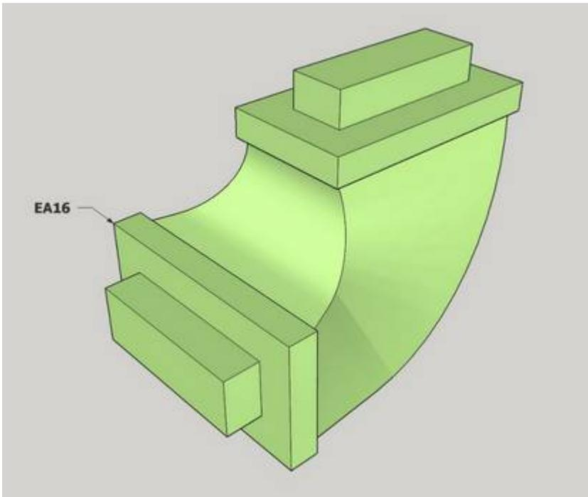
Here's a closer look at EA16. The studs that fit the ID of the tubing (Evergreen #257) may require a swipe with emery board as I said earlier – the dimensions of Evergreen tubing is at best nominal .. they can vary by a few thousandths either way.
