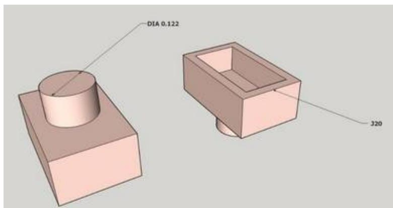
To connect the tubing to the HVAC unit we are using a J20 joiner. There are an assortment of joiners allowing you to connect tubing to any flat surface. In the case of the J20 there is a small stud on the back side. This fits a 1/8" hole you drill
