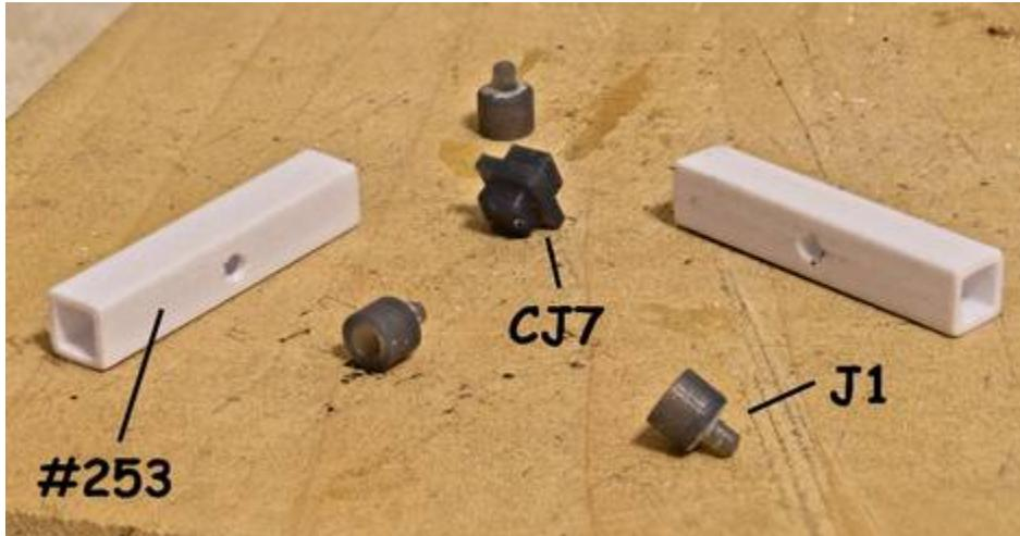
I skipped ahead to the main body of the ducting. Rusty Stumps supplies a 2" length of #253 tubing (3/16" sq.)
