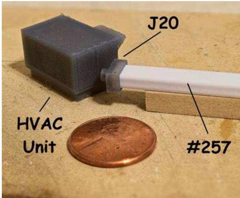
Here we can get a close look at the HVAC unit. Note the little 'nibs' on the unit. These are the remains of the support structures used during printing and need to be removed with sandpaper such as emery boards.
